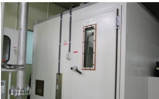
EMC shield room
