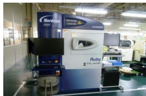
3-Dimensional X-ray inspection equipment
