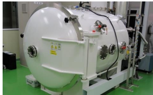
Thermal vacuum chamber
