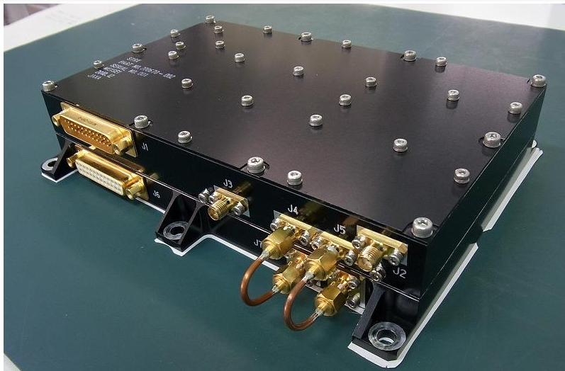
Upper section : USB transceiver unit Lower section : QPSK transmission unit
